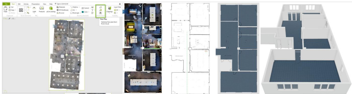
Figure 7: Floor plan generation from a point cloud
