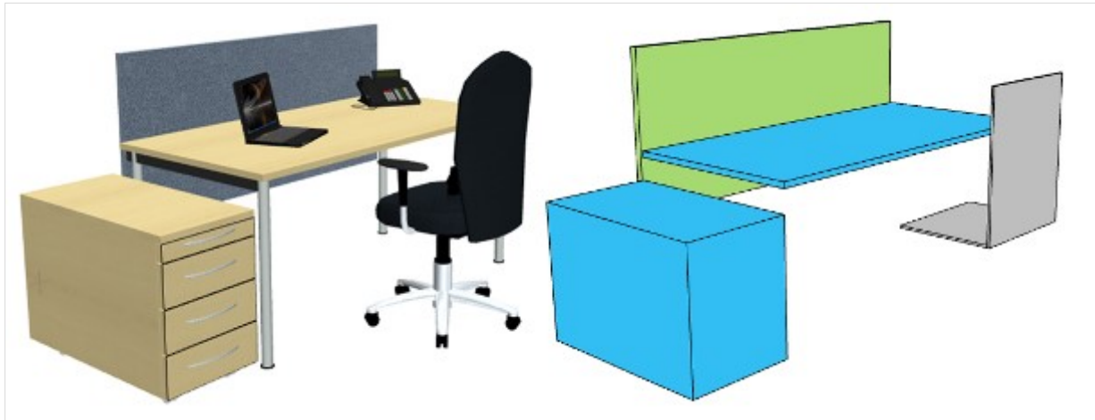
Detailed 3D design (left) and simplified acoustic representation (right)
