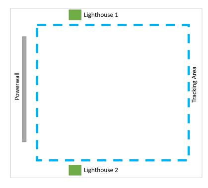
The prerequisite for the use of the interactive Virtual Reality wall is the correct positioning of the HTC VIVE base stations that should be found to the left and right of the Powerwall. In addition, ensure that the room calibration from the *SteamVR* is also valid.
